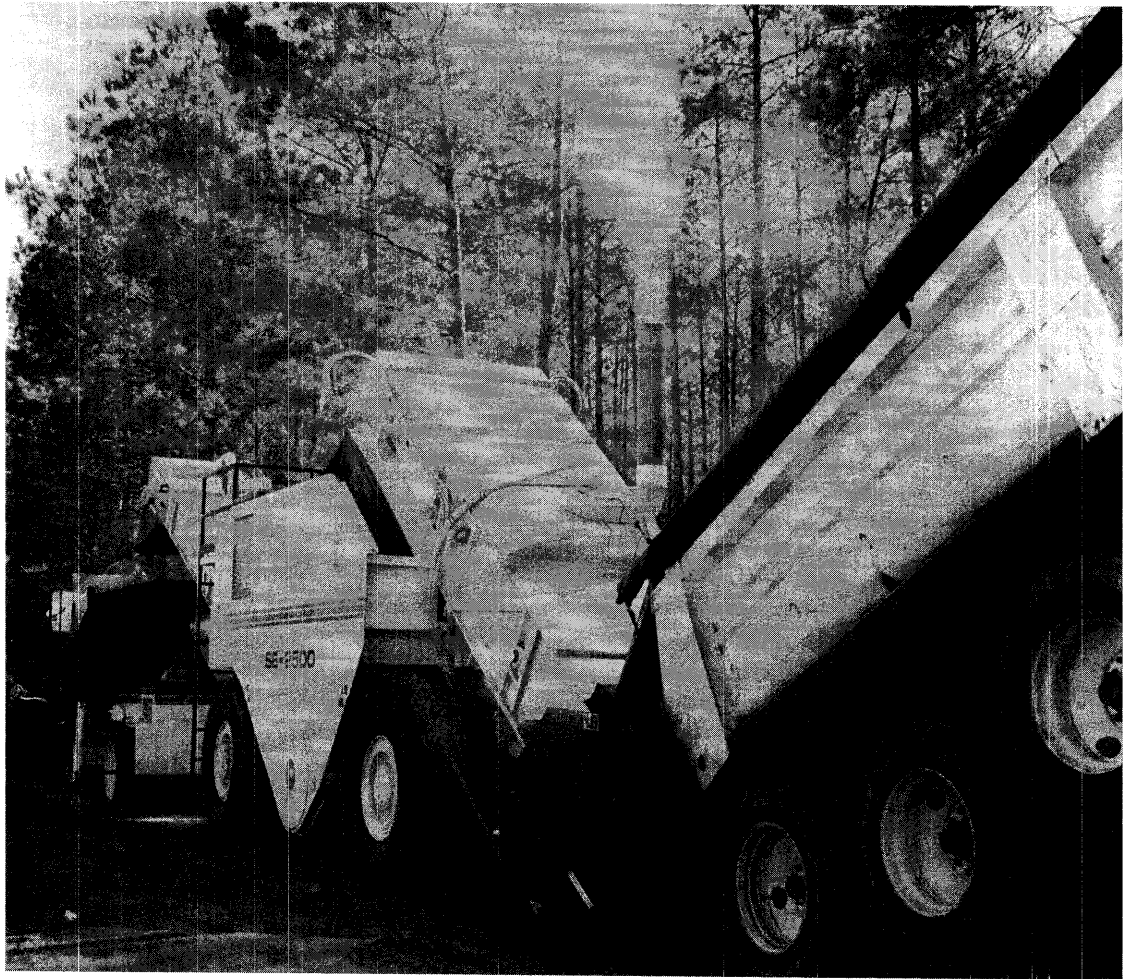
Figure 8-6 Material transfer vehicle feeding an asphalt paver. (Courtesy of Roadtec, Inc.)
